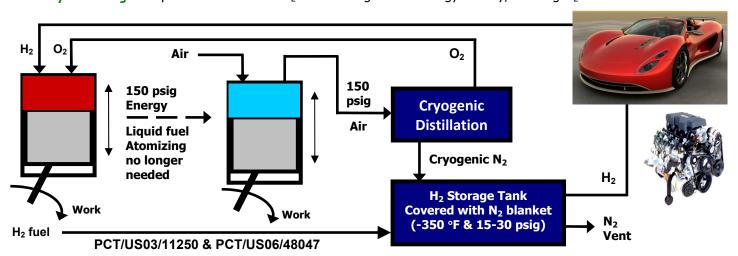
Combustion of pure  $H_2$  with pure  $O_2$  improves combustion chamber effectiveness by 80%; as otherwise, air is only 20%  $O_2$ ; yet, is 80% nitrogen  $(N_2)$ . Ironically and nicely, the amount of energy required to separate air is near that of the backpressure required to combust liquid hydrocarbon fuels; therefore and in comparison to the traditional combustion engine, a  $H_2O_X^{TM}$  Engine produces pure combustion  $O_2$  for fee.
